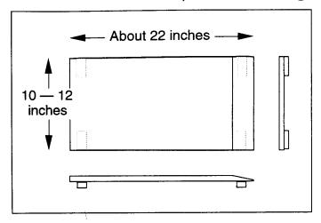
of the platform on the rollers should any doubt about it's use remain. The platform goes under the belt and is placed so that it's rear edge is roughly under the bottom bracket of the bike. The groove shown on the platform in the drawing is the way it looks on my hastily built original. The platform may rattle at some speeds. If so, just pad the contact areas. I hope you find these ideas useful.
